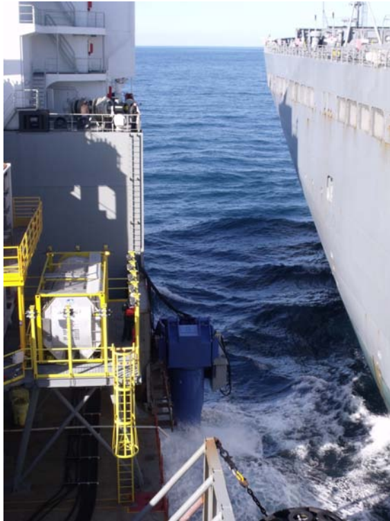
Figure 9: View forward during sea trial, vessels are in position for a crane transfer, and their relative watch circle is 1.5m
