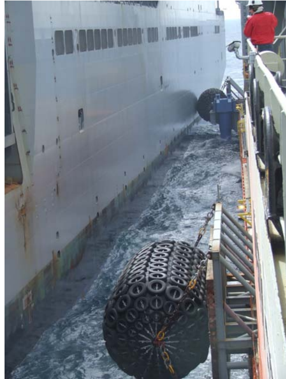
Figure 10: View aft during sea trial, vessels in position, aft fender touching, underway at 3.7 knots
