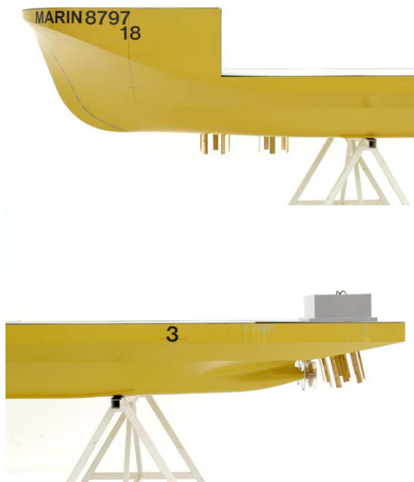
Figure 1 – Photographs of Bow and Stern of Mighty Servant 3 Equipped with Voith Schneider Propellers
