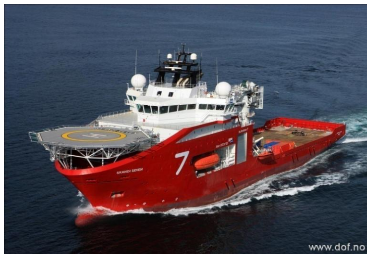
Figure 1 This 120 meter long construction support vessel (CSV) named Skandi Seven is a typical vessel for the discussed operations
