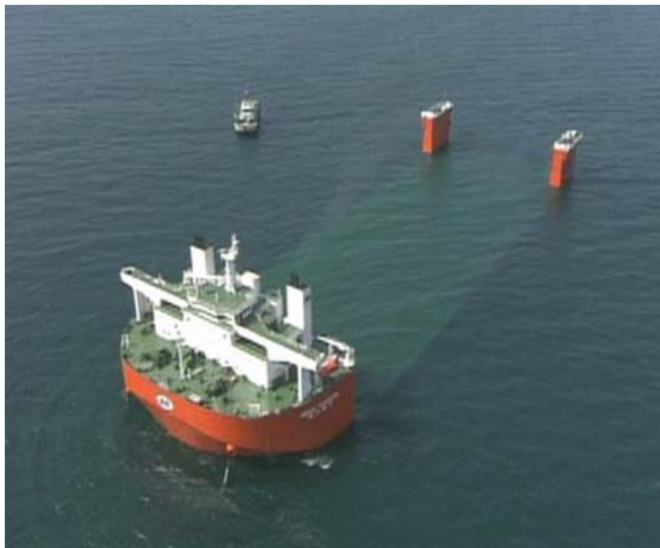
Figure 3. Heavy Lift Carrier Submerging
