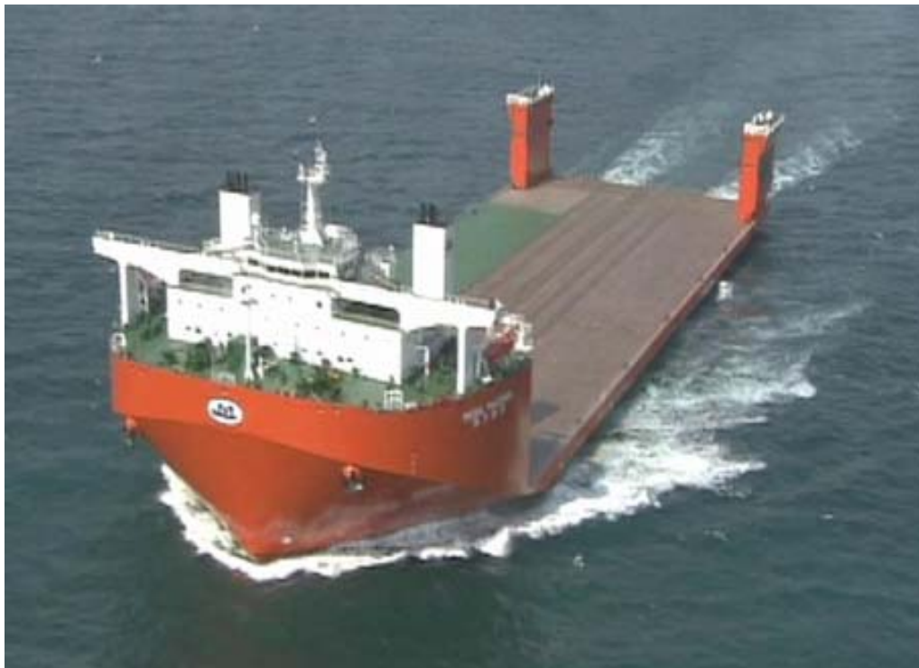
Figure 2. Heavy Lift Carrier; TPI MEGA PASSION
