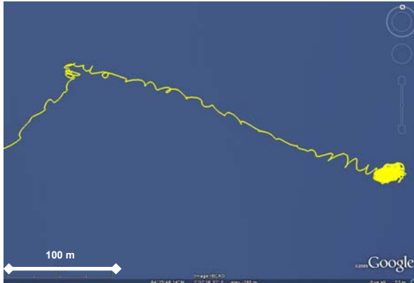
Figure 8: Antenna movement on Bourbon Topaz offshore due to wave motion.
