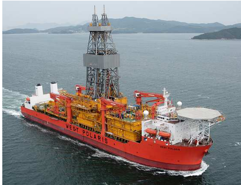
Figure 1. Sixth generation drillship equipped with a dual derrick
