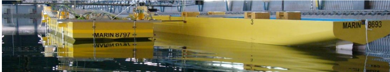
Figure 9: Photograph showing the two vessels in side by side arrangement, where Mighty Servant 3 (the left vessel) is equipped with wave height sensors to measure the wave feedforward force.
