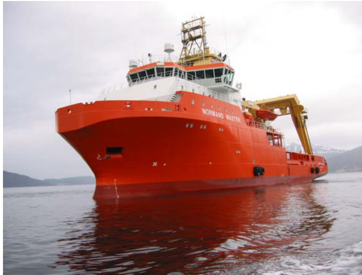
Figure 1 – DP2 Multifunctional Anchor Handling & Tug Supply Vessel (Photograph courtesy of Solstad)
