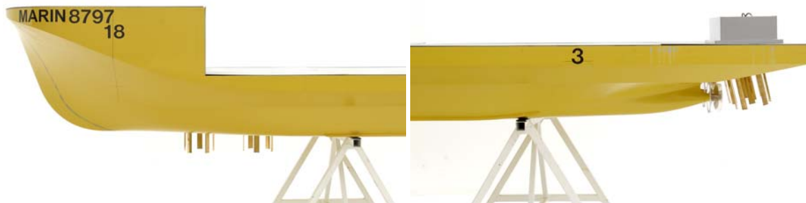
Figure 3: Photographs with fore and aft ship of Mighty Servant equipped with Voith Schneider propellers
