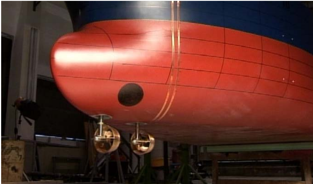
Figure 4 Forebody of model showing two azimuth thrusters and marking of bow tunnel thruster position.
