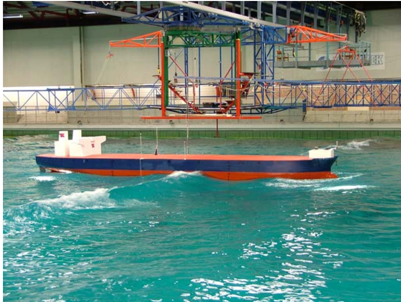
Figure 2 DP Offshore Loading in Marintek’s Ocean Basin Laboratory. The Teekay model is controlled by an “off the shelf” Kongsberg DP system.
