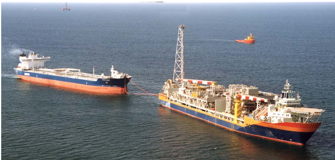
Figure 3 DP Offshore Loading at Aasgard A field in the North Sea.
