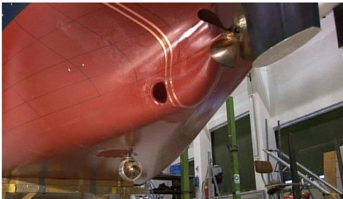
Figure 5 Aftbody of single screw hull showing azimuth thruster, stern tunnel thruster, main propeller and rudder.
