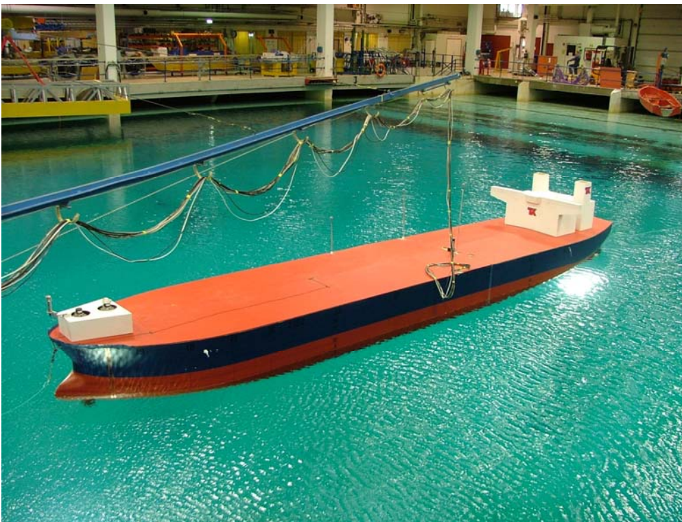
Figure 10 The 10 meter long model ready for DP testing in Marintek’s Ocean Basin. The model is controlled by an “off the shelf” Kongsberg DP system.
