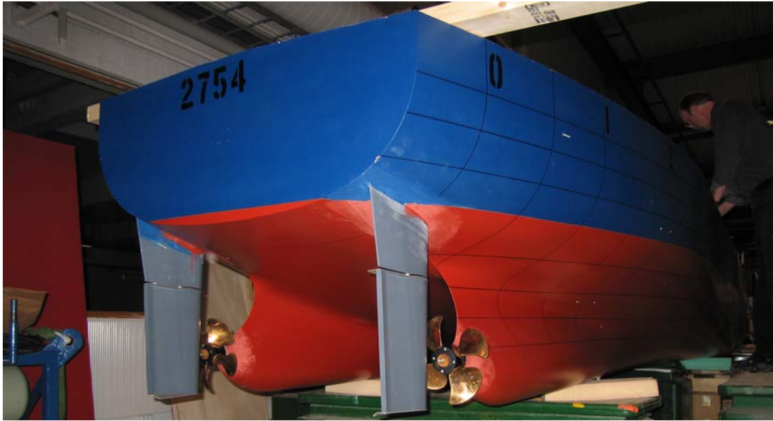
Figure 6 Aftbody of twin screw tanker where skegs, propellers and rudders can be seen. The aft azimuth thruster is located at centre line between the skegs.
