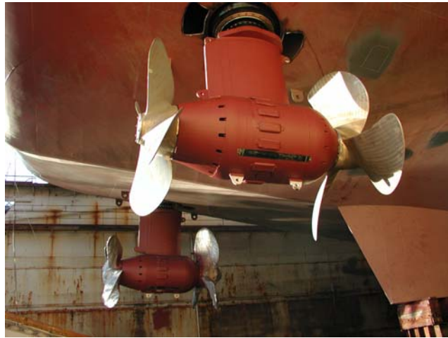
Figure 2 Steerprop 35 CRP installed in a ROV vessel
