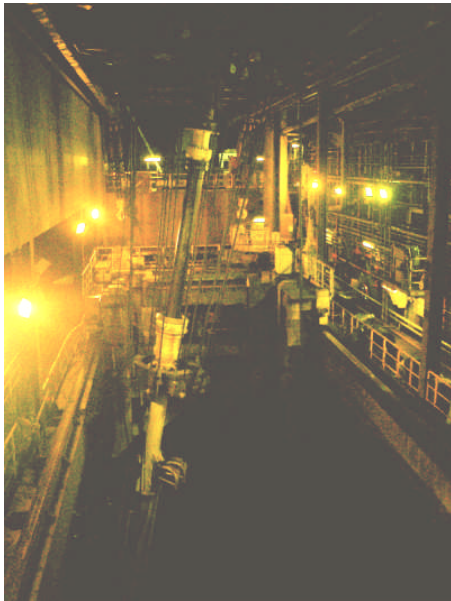
Figure 3 - Wide Moonpool Allows Large Upper Angle
