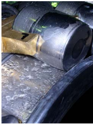
Figure 2.3. Damaged raceway, result of bad lubrication
