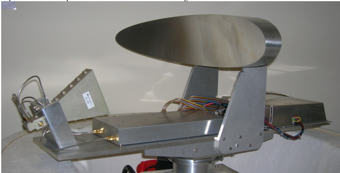
Figure 1: The RadaScan sensor with radome cover removed
