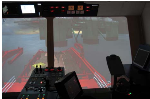
Figure 14. Visualisation in 3D of complete anchor handling operation at the Offshore Simulator Center (OSC) in Aalesund, Norway.
