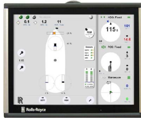
Figure 4. New range of graphical displays, here with a Poscon DP user interface.
