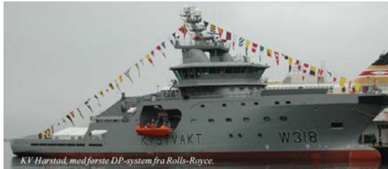
Figure 13. Norwegian Cost Guard vessel, K/V Harstad. Rolls-Royce UT 512 design with Poscon DP system.
