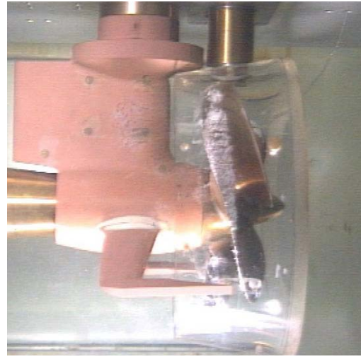
Figure 11 Thruster with design propeller at V_{tip} = 46 m/s, T = 17.5 tons
