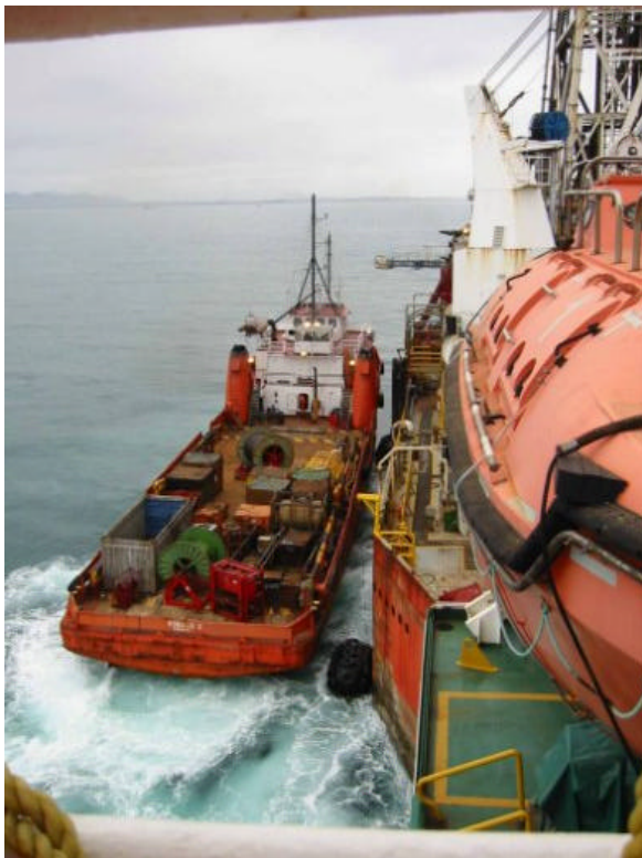
Figure 20, Relative DP operation between two moving vessels.
