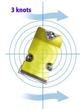
Figure 1 In station keeping, the system's ability to withstand currents is limited by the propulsion power of the WROV
