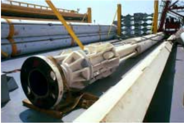
Figure 9. Riser Joints and Termination Joint
