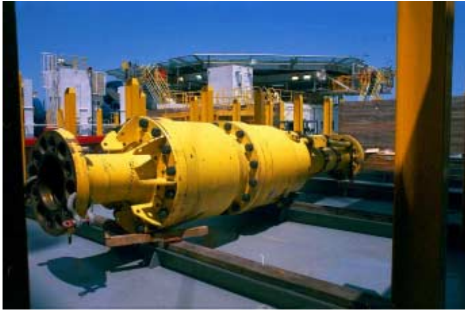
FIGURE 7. Riser Gas Handler
