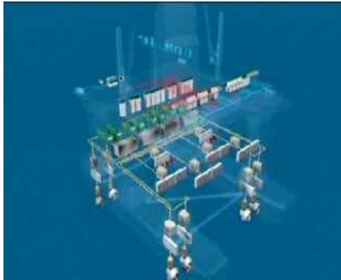
Fig. 1: The electric power and thruster system is an integral part of the overall station keeping system for a semi submersible rig.
