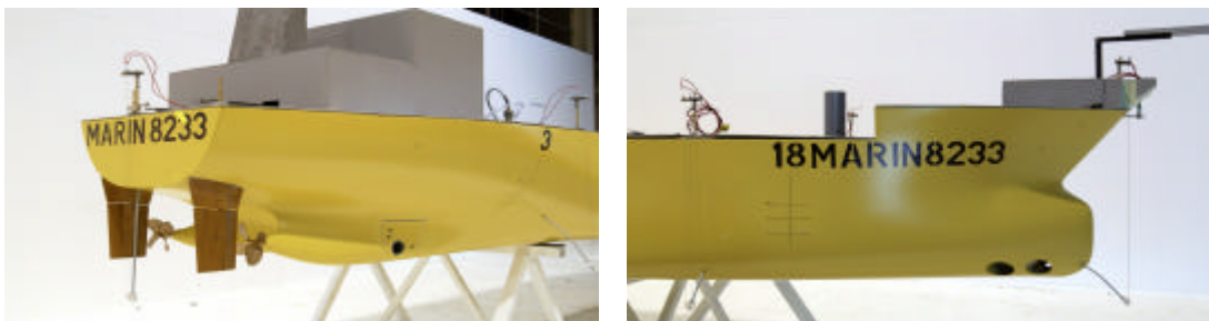
Fig.2: Stern and bow thruster arrangement on the shuttle tanker model
