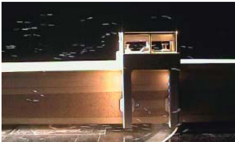
Figure 13 - Test with Helium Bubbles
