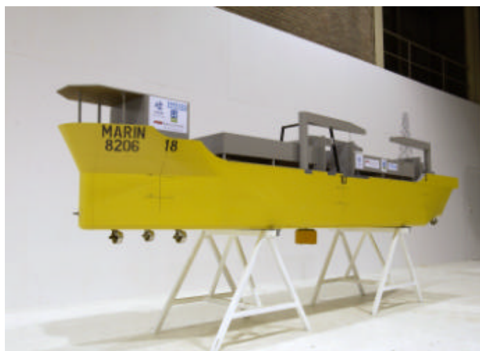
Figure 5. DP FPSO model with disconnectable buoy
