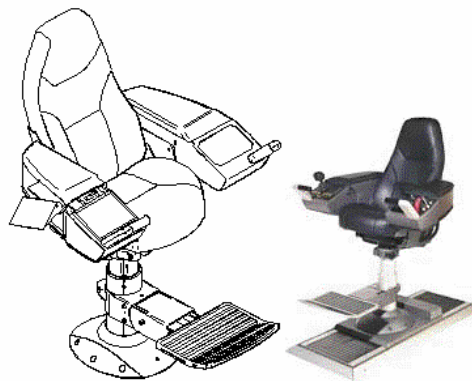
Figure 6 - Chair for installation of levers in armrests (AS Sorlandets Aluminiumsprodukter)
