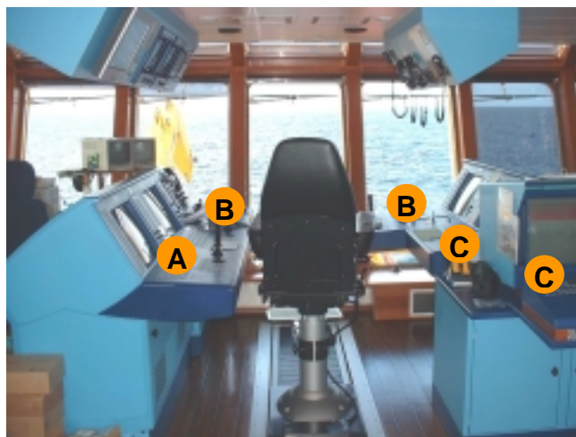
Figure 1 - Typical PSV Aft Bridge built for a single operator with equipment for an additional vessel automation operator (A: Dual DP, B: Manual Thruster/Propulsion Control, C: Vessel Automation)
