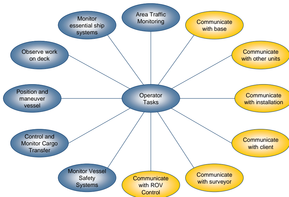
Figure 3 - Operator tasks executed from the workspace on the aft bridge during normal operation. Tasks shown with yellow background are communication tasks.
