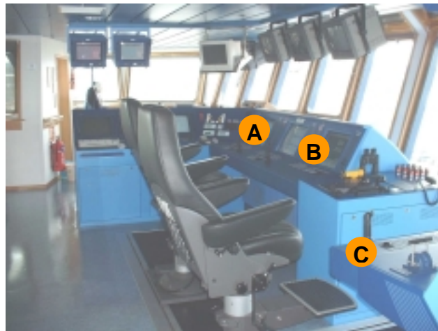
Figure 2 - PSV aft bridge with two operator positions, but often manned by one person. A (Vessel Automation), B (Dual DP), and C (Manual Thruster / Propulsion Control and Joystick).
