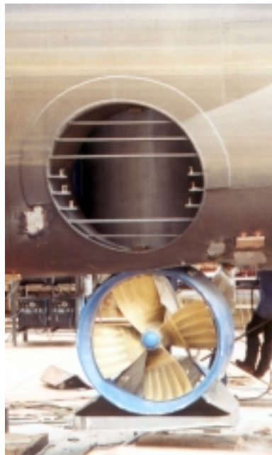
Figure 2: Retractable combination thruster
