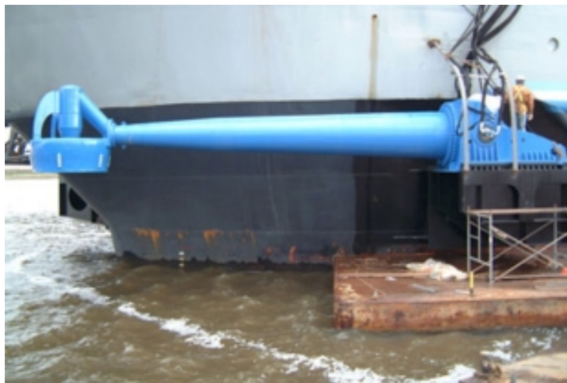
Figure 16: Propeller Ventilation - DP Stem
