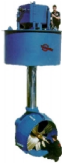
Figure 6: Retractable Azimuthing Thruster with Hydraulic Drive
