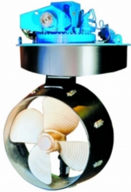
Picture 2: Twin-prop (CRP) Contaz-unit
