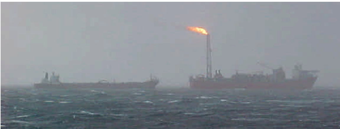
Figure 4: Terra Nova FPSO offloading to shuttle tanker offshore Newfoundland
