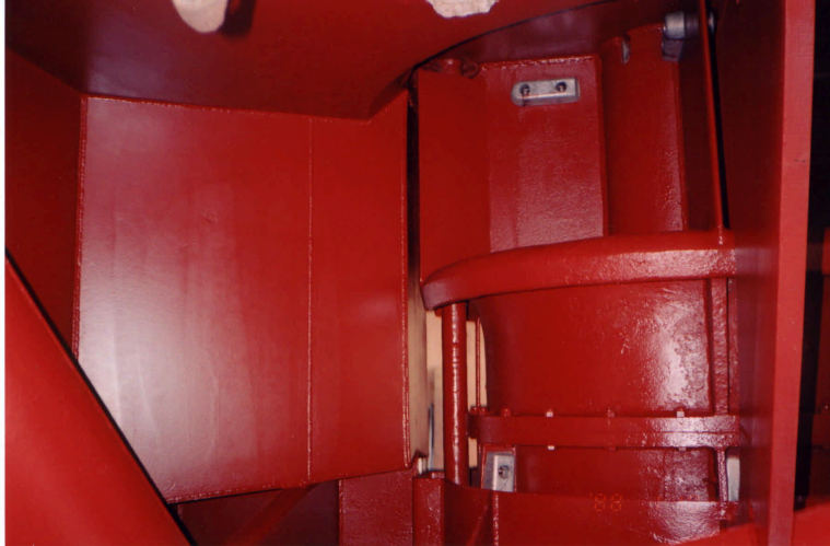
Figure 10: “Wedge-Bulkhead” Steering Shaft Enclosure
