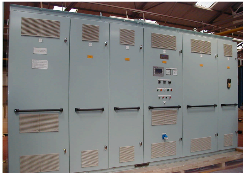
Figure 10 - 2400kW MV3000LC PWM Converter Construction
