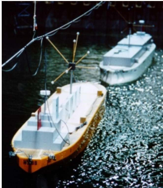
Figure 6. Tandem Moored Tanker Model Test in Offshore Basin
