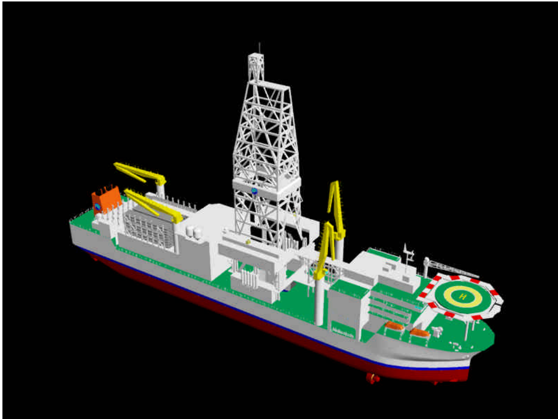
Figure 1 General arrangement and 3-D model of the OD21 drillship
