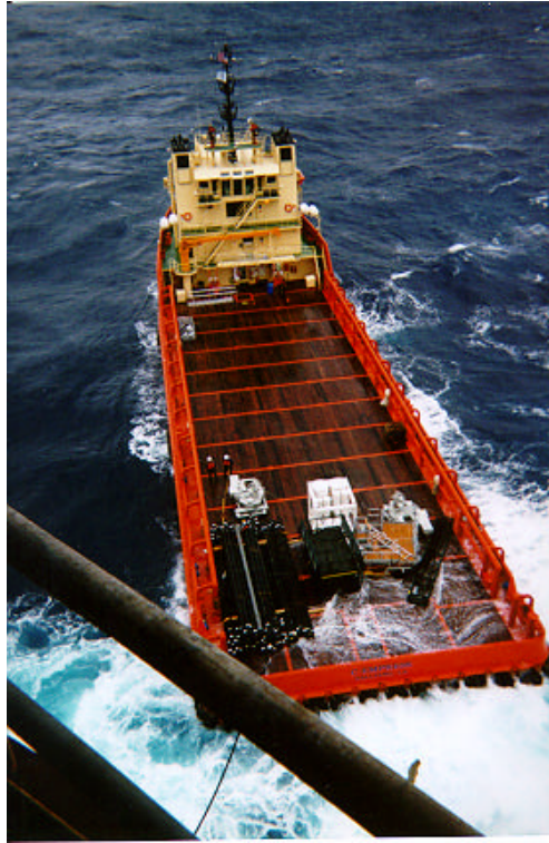
Figure 10. The C-Empress transferring fuel to the URSA TLP under DP control.
