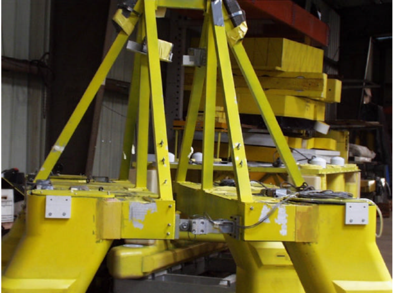
Fig. 7 Sectional Load Measurement Technique on the Hull of a Moored Floating Structure in a Seakeeping Test
